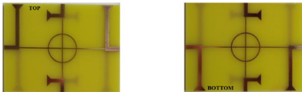
Fig. 7. Fabricated four element MIMO antenna in [40].
